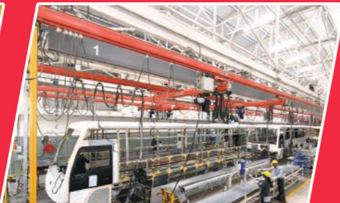
STRUCTURE MAKING USE OF JIGS & FIXTURES
