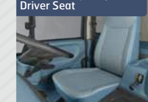
Mechanically Suspended Driver Seat
