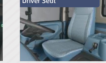
Mechanically Suspended Driver Seat
