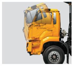
Fully suspended cabin with hydraulic tilt mechanism
