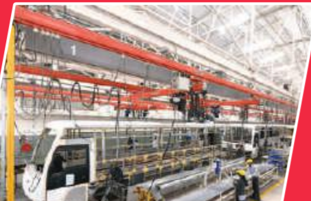
STRUCTURE MAKING USE OF JIGS & FIXTURES
