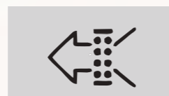
Air Filter Restriction Indicator
