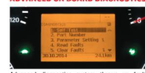
Advanced diagnostics system throws up fault indicators to the driver in the form of visual signals, messages and alarms to check for probable causes and take corrective action.
