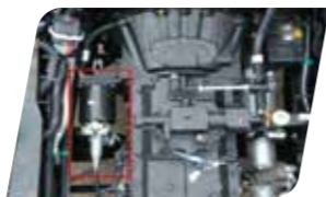
ET35 Transmission with Clutch Booster
